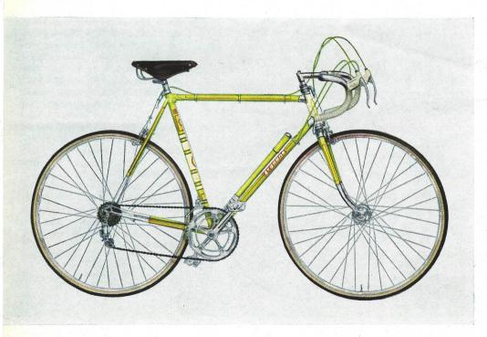
Frame: Special double butted tubing size 21-34" or 23-34" - Chrome plated lugs. Chrome plated front and rear fork ends - Wheels: Fiamme alloy sprint rims with conical bushes. Butted rustless spokes. Pirelli best quality tubular tires - Brakes: Universal Center Pull with rubber hooded levers - Saddle: World best Brooks B-17
